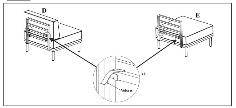
Position Seat Cushion (E) into position as shown, ensuring the zipper faces down. Secure using the preattached Velcro straps to the bottom rail of the Backrest Frame (B). Position the Back Cushions (D) into position as shown, ensuring the zipper faces down and the angles surface faces to the front. Secure using the preattached Velcro straps to the mid rail of the Backrest Frame (B).
