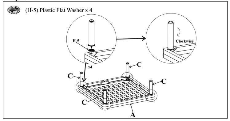
Using a second person to assist you, place Seat Frame (A) upside down onto a padded, non-marring surface. Position the corner Legs (C) on Seat Frame (A) as shown.
