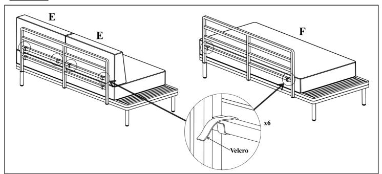
Position Seat Cushion (F) into position as shown, ensuring the zipper faces down. Secure using the preattached Velcro straps to the bottom rail of the Backrest Frame (B). Position the Back Cushions (E) into position as shown, ensuring the zipper faces down and the angles surface faces to the front. Secure using the preattached Velcro straps to the mid rail of the Backrest Frame (B).
