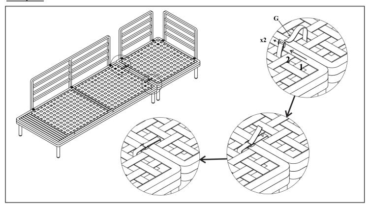
If joining with with a partnering piece, place both assemblies side by side in your desired orientation. Secure together by threading two provided Strap Connectors (G) through the webbing and around each frame, one toward the front of the frames and one toward the back. Tightly secure.
