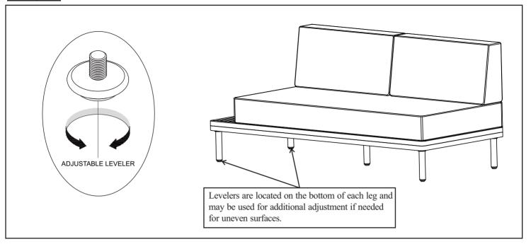
Assembly is now complete and the product is ready for use. Adjustable levelers are located on the bottom of each leg and may be adjusted by turning outwards, counter-clockwise to help account for uneven surfaces. NOTE: Hardware may loosen over time. Periodically check that all connections remain tight and adjust as needed.
