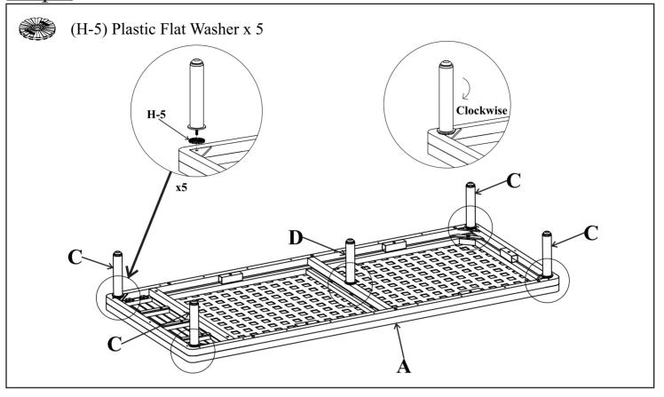
Using a second person to assist you, place Seat Frame (A) upside down onto a padded, non-marring surface. Position Center Leg (D) and the remaining corner Legs (C) on Seat Frame (A) as shown. Note, the Center Leg (D) is slightly shorter than Legs (C). Position the Plastic Flat Washers (H-5) between the legs and the seat frame and tighten by turning clockwise. DO NOT OVER TIGHTEN.
