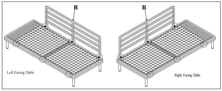
Each component of this collection is designed to be both left and right facing. There are two sets of holes that will accept the backrest. Be sure to decide on your desired orientation before proceeding.
